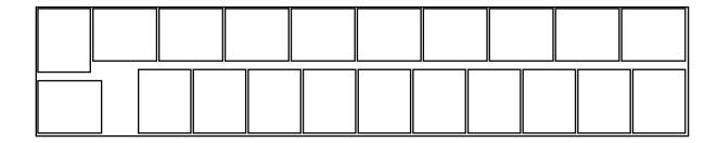
Layout 2:21 pcs of standard pallets fit in a 40ft container
